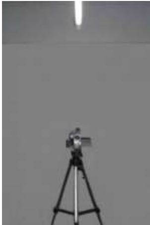
The photo on left shows full-spectrum (FS), daylight fluorescent tube – ceiling-mounted. Camera and light are in line facing the subject.
