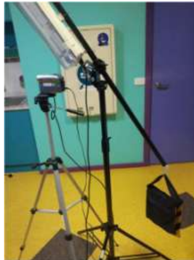
Photo on left shows (FS) fluorescent light tubes mounted on a stand. This type of lighting is quite bright and suitable in a large room – as seen here.
