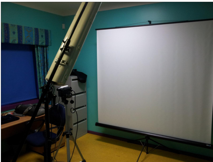
This photo shows FS light mounted on stand projected towards a plain background screen. This is an excellent set up. The light is centred with, and angled towards, the screen. Some users like to angle the light forwards at about 35 degrees from the vertical. A distance of about 2 metres is recommended between the screen and the front of the light. The camera is positioned in front of, and in line with, the light.
